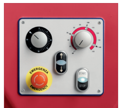
Pannello inverter con sollevatore automatico Control panel with inverter and automatic lift
